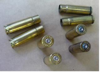
Both pictures above showing fired 'high-velocity' cases on the left, and fired 'subsonic' cases on the right.
